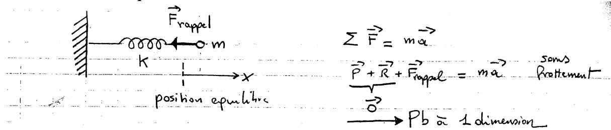
$$m \ddot{x} = F_{Frappe} \rightarrow m \frac{d^2x(t)}{dt^2} \vec{e}_x = -Kx \vec{e}_x$$
